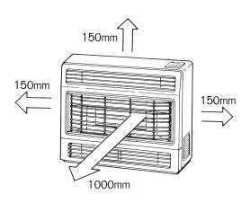
Do not allow curtains or other flammable materials to come into contact with the heater.
