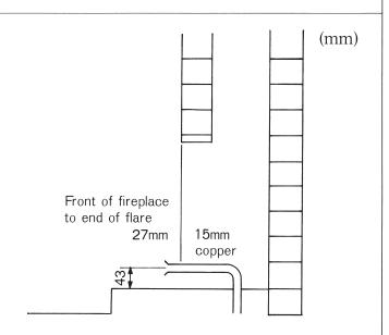
DON'T FORGET TO PUT FLARE NUT ON TUBE BEFORE FLARING.
