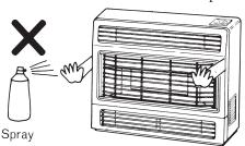
The pilot could also ignite the gas from an aerosol.
