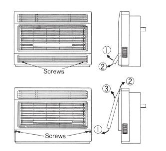
ENSURE THAT REMOVAL AND REPLACEMENT OF THE BOTTOM PANEL IS NOT OBSTRUCTED BY CARPET ETC.
